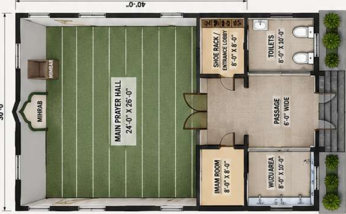
DIMENSION PLAN (GROUND FLOOR)
